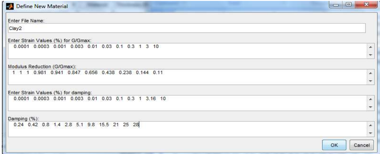
Figure 4 Example inputs for “Define New Material”
