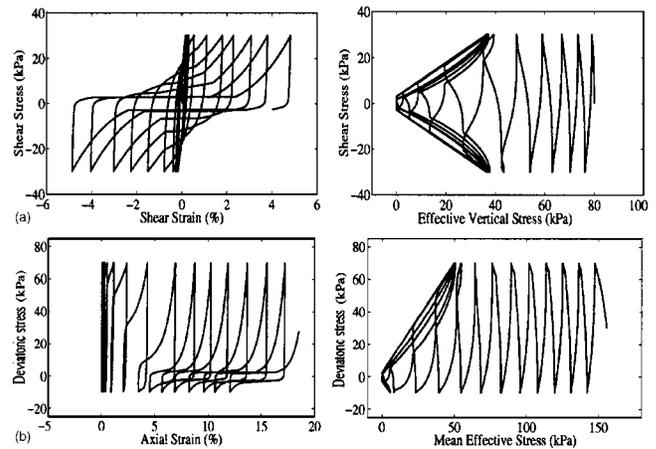
**Fig. 5.** Model simulation of stress-controlled, undrained cyclic shear loading: (a) without and (b) with static shear stress bias (Parra 1996; Elgamal et al. 2003)
